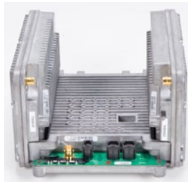
MTR 2000 Control Exciter Receiver Assembly
